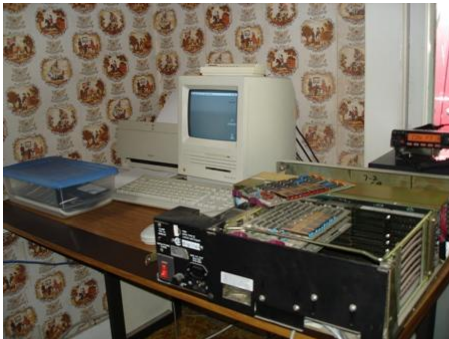
This is a photo of the Macintosh SE hooked up to the pdp-11
