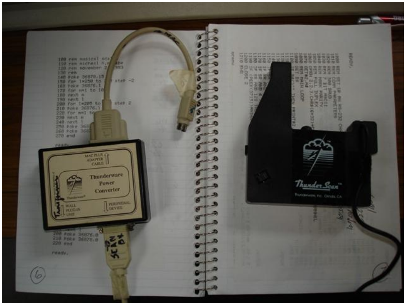
The Thunderscan Cartridge and Association Electronics.
