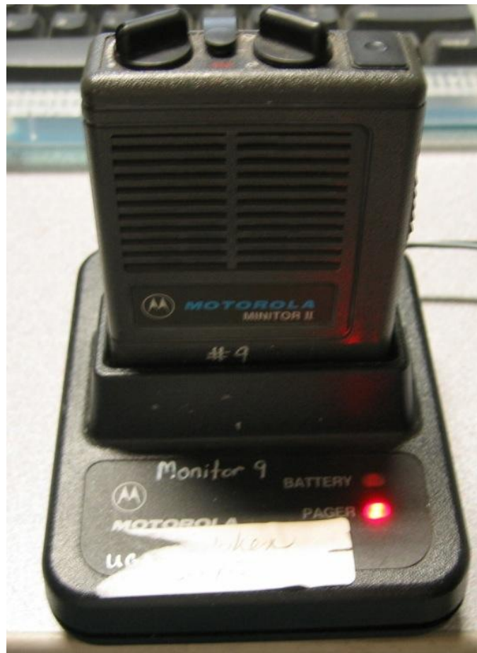
Clunky, but still useful -- this second-generation tone-and-voice pagers are used to alert firefighters and EMS workers of emergency calls. This example dates from 1985.
