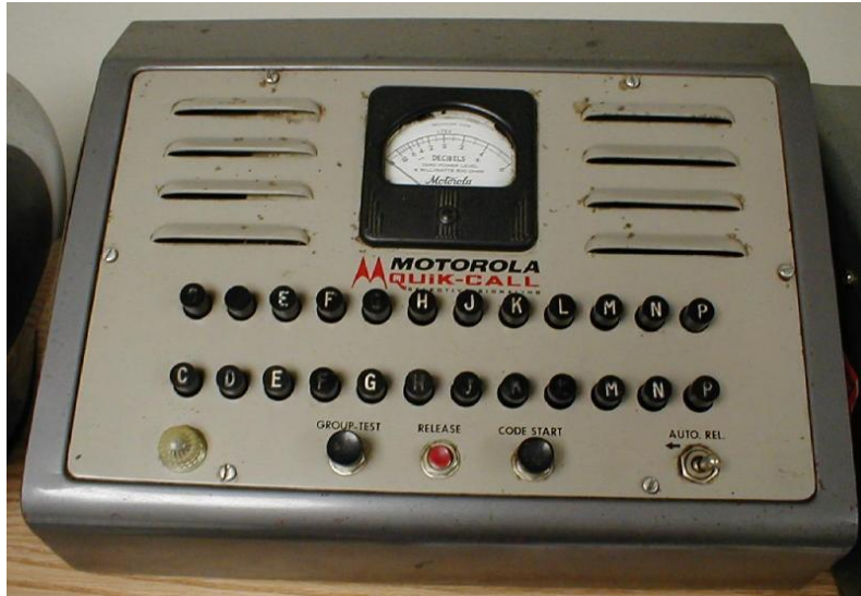
An "antique" Motorola Tone Encoder used to activate tone-alert monitors, pagers, and fire sirens. It produces a unique sequence of dual tones that are similar to DTMF.
